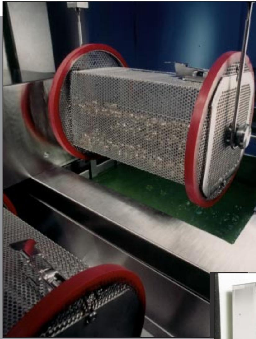
**The best way to clean small parts which tend to nest, cup fluids or have fine blind holes**
